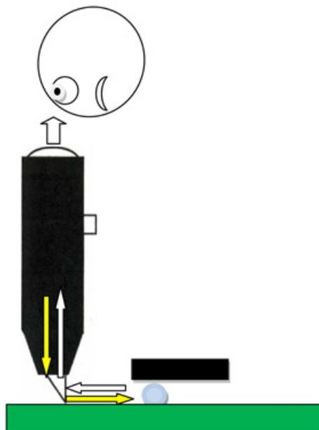
The sensor prism is by special glass, and the tip of the prism is thin, it should be operation with carefully.
